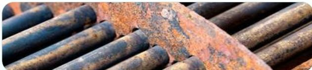
A water softener must be used, along with a "dispersant" chemical that should keep any salts or solid matters in "loose" form – to be drained out by blowdown system. And the corrosion problem in the boiler is gravely serious! Dissolved oxygen in water must be removed in order to prevent reaction on metallic surfaces, thus rusting. An "oxygen scavenger" is absolutely a must.
