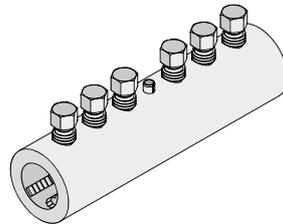
To install; slide the rebar ends into the coupler. A stop-pin is located at the middle of the coupler. Turn the screws in as far as possible. While screwing in the shear-off screws, the special hardened tip digs into the rebar, simultaneously pressing it against the serrated runners. This creates a positive connection between screw-tips and the rebar and between rebar, serrated runners and inner surface of the coupler.
