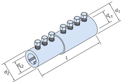
HALFEN Reinforcing coupler type MBT RDZ 16/14, transition coupler for connection of reinforcing steel with different diameters  $d_{s1}/d_{s2} = 16/14$  [mm].
