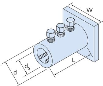
HALFEN Reinforcing coupler type MBT EV 25, head coupler for reinforcing steel diameter  $d_s = 25$  mm.
