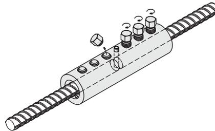
If the pin is missing, mark half the of the coupler length on the rebar and slide the coupler on the rebar up to said mark.
