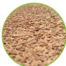
Micro exposure. Exposure depth approx. 1.5 mm
